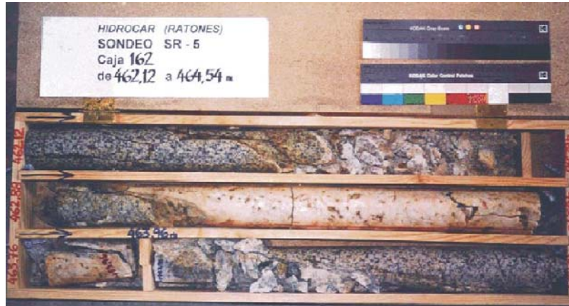
Figure 19. Core from borehole SR5. The white zone corresponds to an ankeritic dyke at around 463 m depth.
