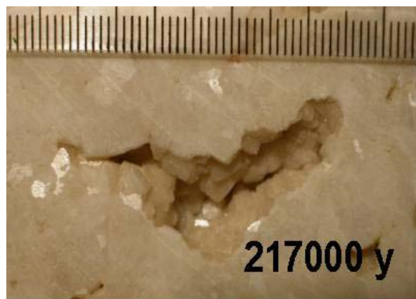
Figure 20. Examples of carbonate crystals studied in the ankeritic dyke ( \approx 464 m depth). The age is measured from \alpha -spectrometry.
