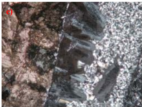
Figure 18. a) View of the fracture fillings (optical microscope) from thin sections: b) and c) carbonates textures d) Visu photograph e) microphotograph of the carbonate, the quartz and the apatite in one section of this fracture filling.
